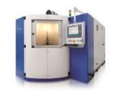
Fig. 3: This test stand by Poppe + Potthoff Maschinenbau produces strong impulses up to 6,000 bar with a frequency between 1 and 30 Hz to check the durability and strength of components under pulsating inner pressure.
