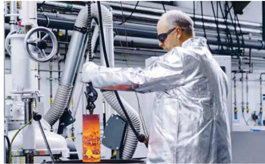
Isabellenhütte machined casts weigh between 1.5 and 3.0 tons. Even small amounts can be melted in the sample furnace.
