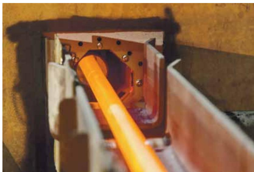
*Sensors generate data. When manufacturing tubes, wire, and steel bars, laser light section sensors measure up to 5,000 contours per second and convert them into a high-resolution 3D model during the production process.*
