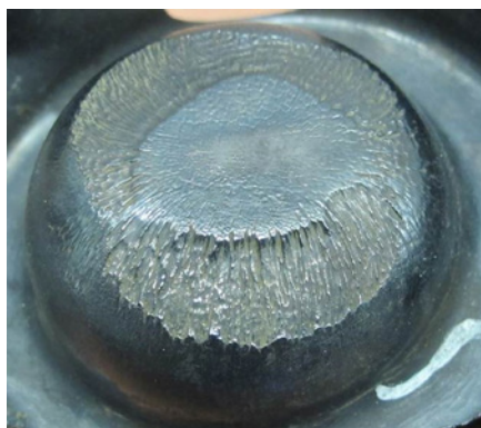
Figure 2: Abrasive wear on a forging die Source: Kind & Co., Edelstahlwerk, GmbH & Co. KG
