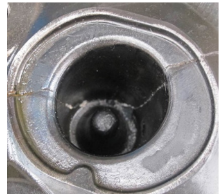
Figure 4: Mechanically induced crack in a forging die Source: Kind & Co., Edelstahlwerk, GmbH & Co. KG
