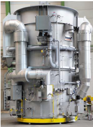
Picture 1: Tenova LOI Thermprocess Ultra low NO x HPH ® Flameless heating hood at thyssenkrupp Hohenlimburg
